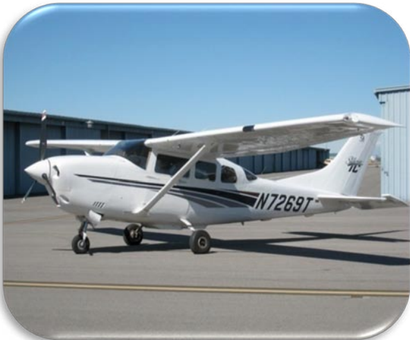
Exhibit 3: The acquisition platform for the Nye County area was a turbo charged Cessna 206. Our 206 has been customized for LiDAR and other airborne sensors with an upgraded power system and avionics. The stability of the Cessna 206 is ideal for LiDAR collection.
