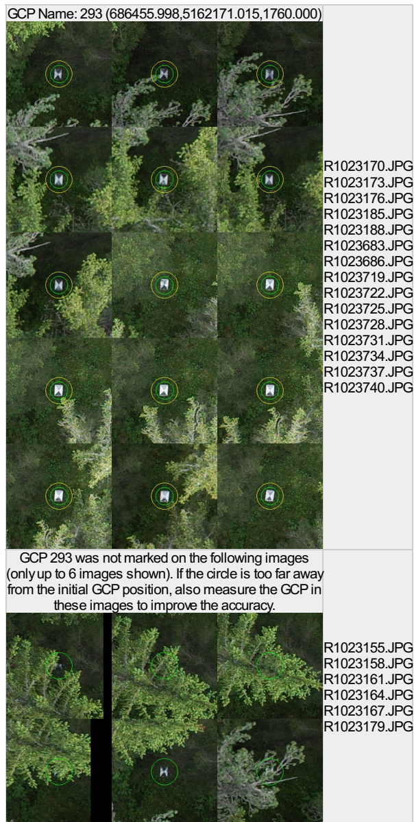
Figure 7: Images in which GCPs have been marked (yellow circle) and in which their computed 3D points have been projected (green circle). A green circle outside of the yellow circle indicates either an accuracy issue or a GCP issue.
